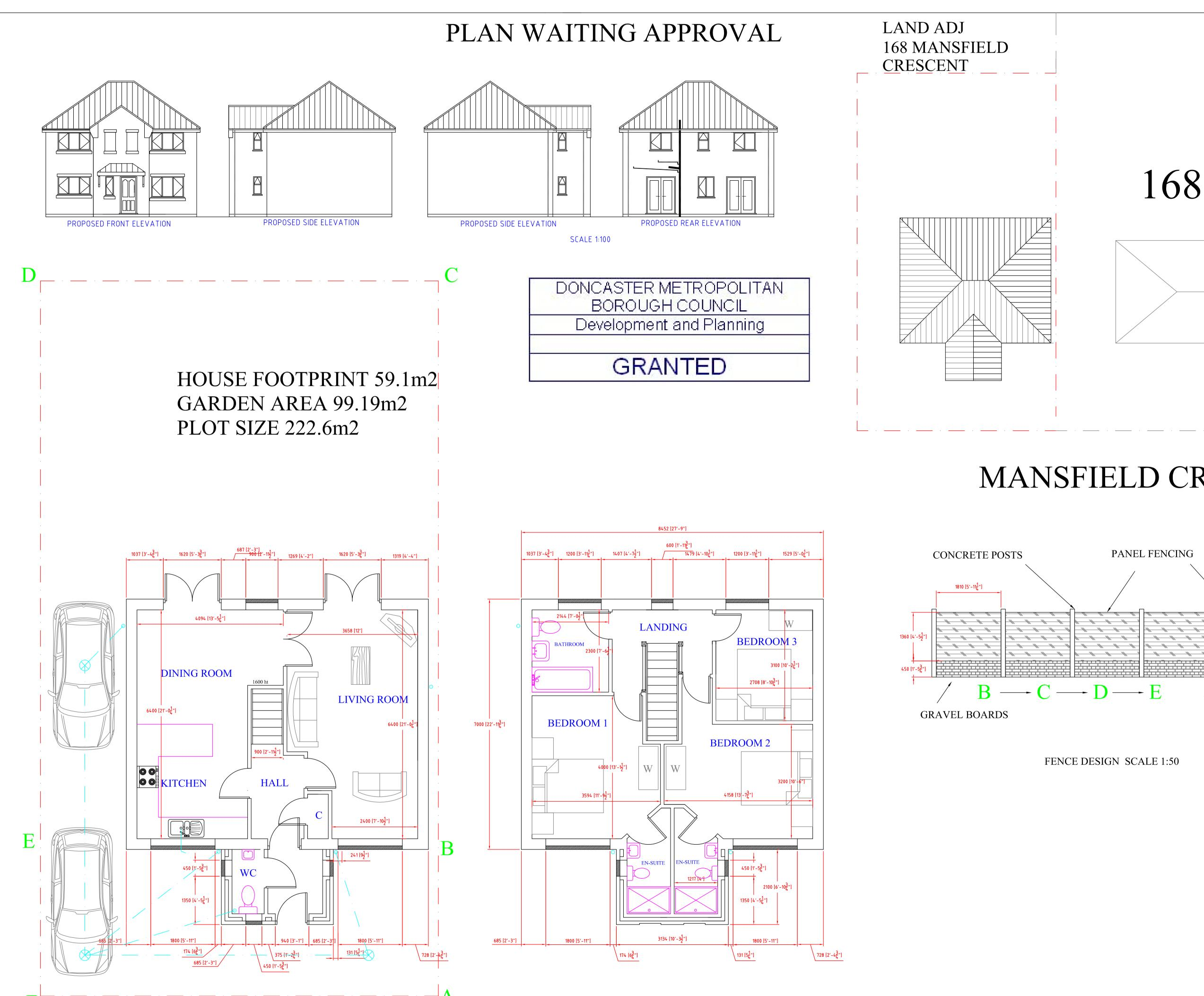
The proposal is to build a 3 bedroom detached house with off road parking for 2 cars All work will be carried out in accordance with Building Regulations and all materials used will be of good quality and to current B.S. specifications.
